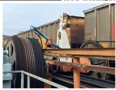
Photo 14: Claw That Holds the Line of Cars while one is Rotated
