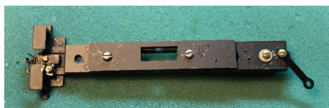
Photo 18: A view of the locomotive frame with couplers mounted.
