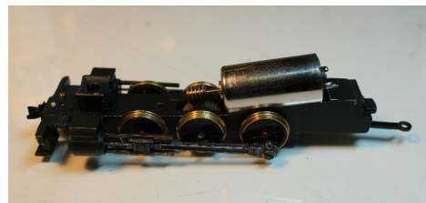
Photo 19: A new can motor installed on the frame.
