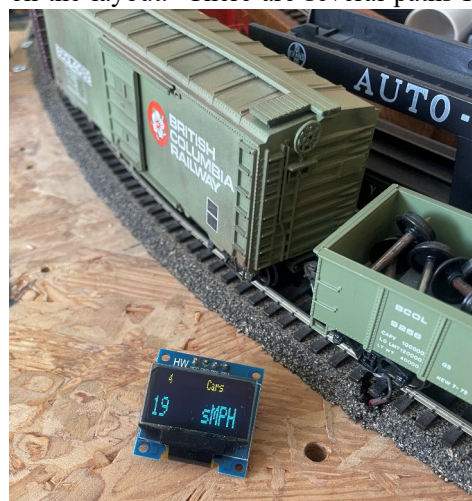
Figure 2: Speedometer/Car Counter Display
