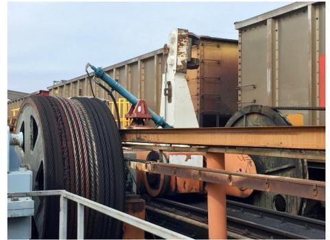
Photo 14: Claw That Holds the Line of Cars while one is Rotated
